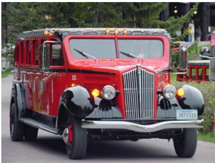
One of The renovated "reds," with slightly wider fenders, slightly smaller tires, and dual tires on the back axle. (Jeff Kuhn photo)
